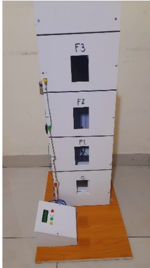
Figure 2. Completed three-floor elevator prototype after demonstration.
